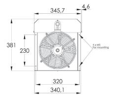
Mounting brackets are compatible with most common nacelle fan heaters.
